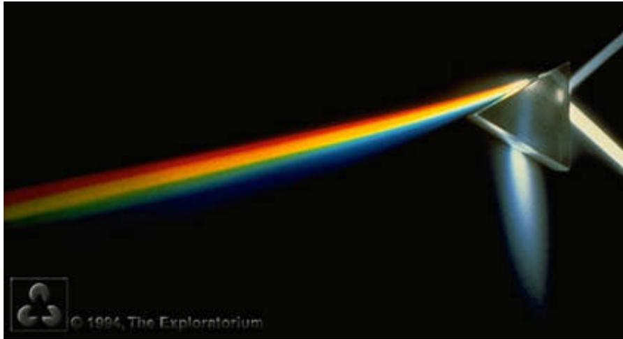
**Figure 3:** White light falling on a glass prism, dispersed into its constituent colors.
