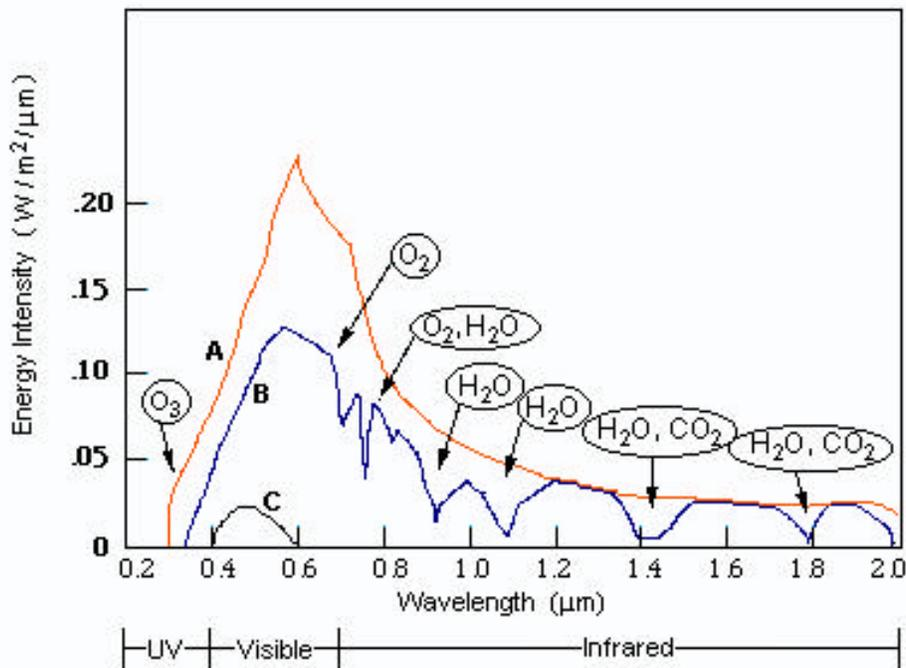
**Figure 8:** Solar spectrum (A) above the atmosphere and (B) near the Earth's surface, with some of the radiation having been absorbed by molecules in the atmosphere. Also depicted is a curve of the spectrum detectable by the eye (C).
